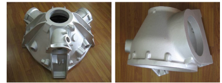
图20 新一代直升机的传动系统机匣 Fig.20 Transmission system receiver of new generation helicopter
